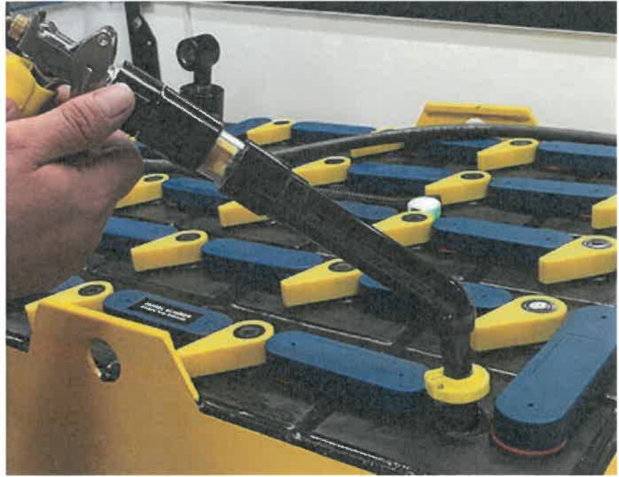
Battery watering gun for lead acid batteries
