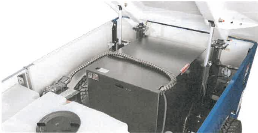
Lithium-ion battery in the Zamboni Model 450
