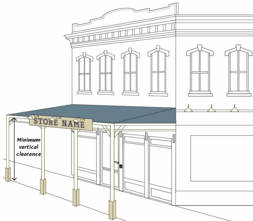
Figure G 2.3.2.8: Awning with Sloping Canopy Roof
