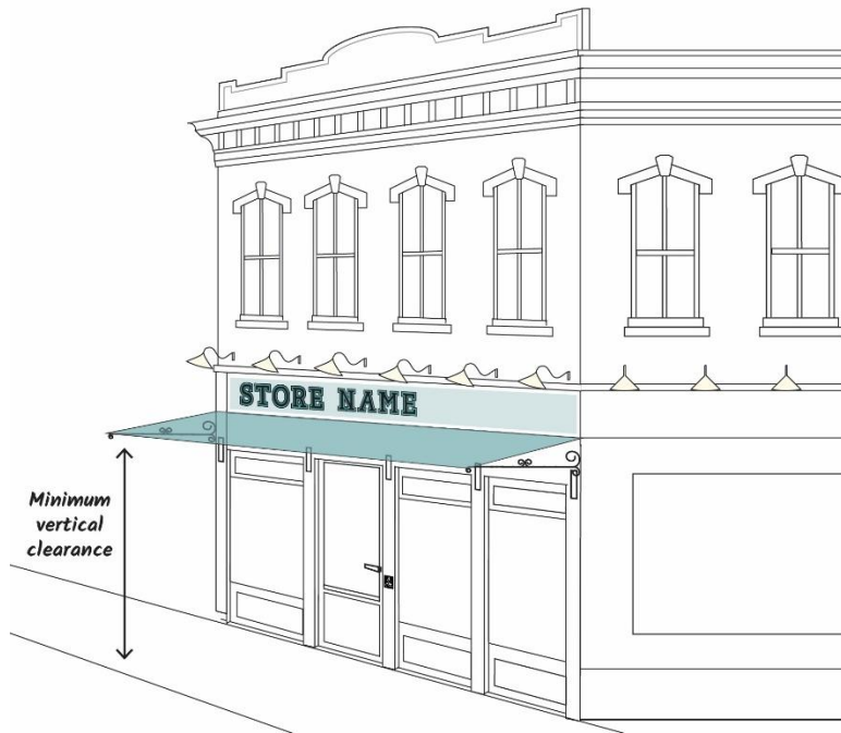
Figure G 2.3.2.2: Awning Minimum Vertical Clearance
