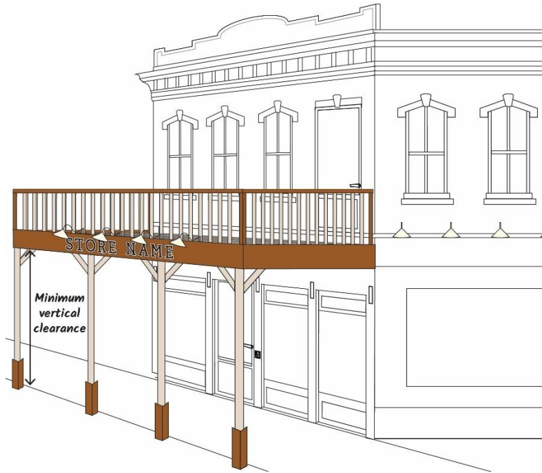
Figure G 2.3.2.6: Accessible Porch with Railings
