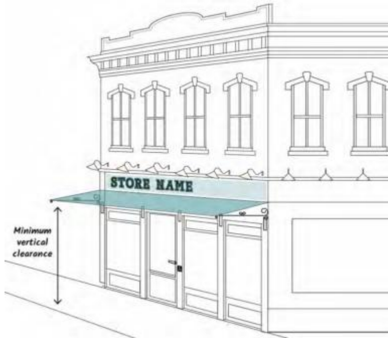
Figure G 2.3.2.2: Awning Minimum Vertical Clearance
