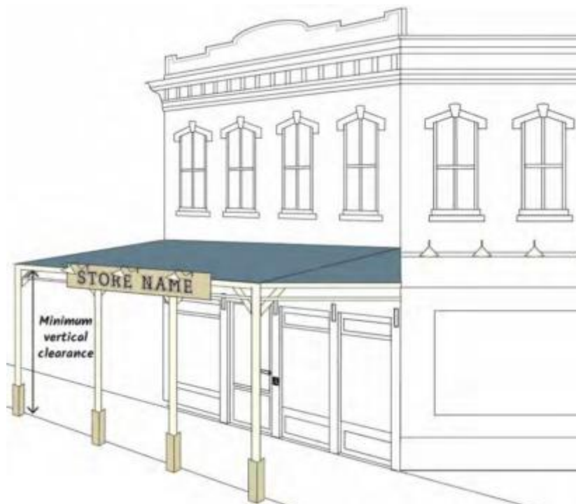
Figure G 2.3.2.8: Awning with Sloping Canopy Roof
