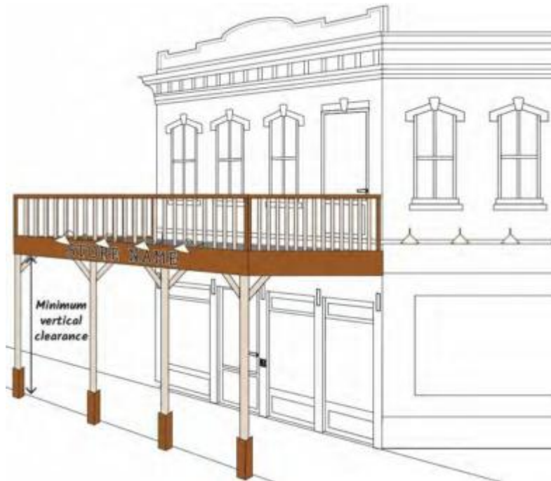
Figure G 2.3.2.6: Accessible Porch with Railings
