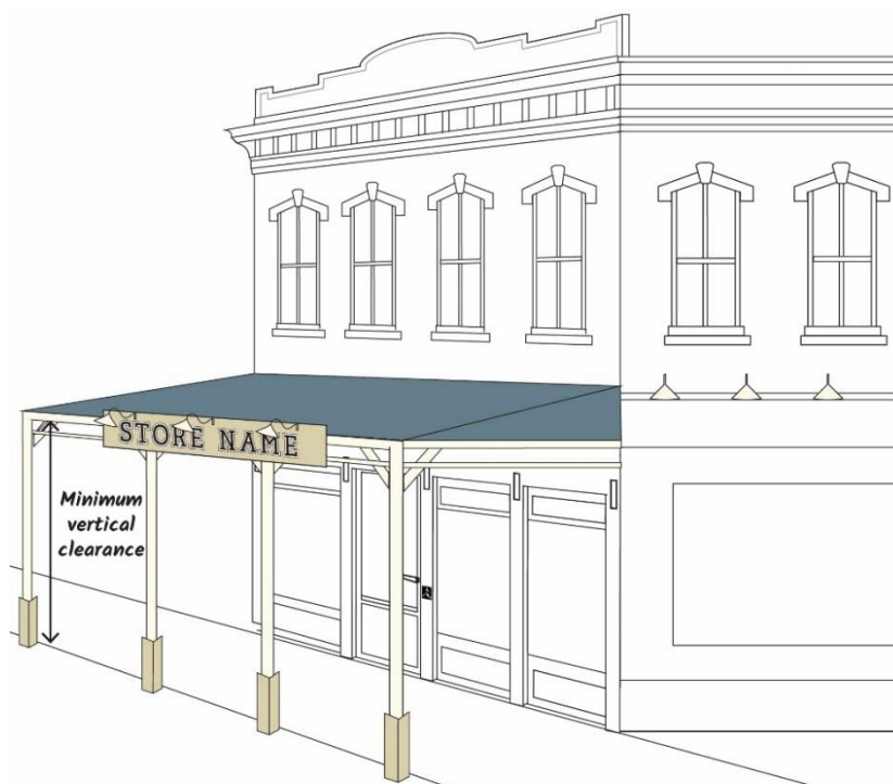
Figure G 2.3.2.8: Awning with Sloping Canopy Roof
