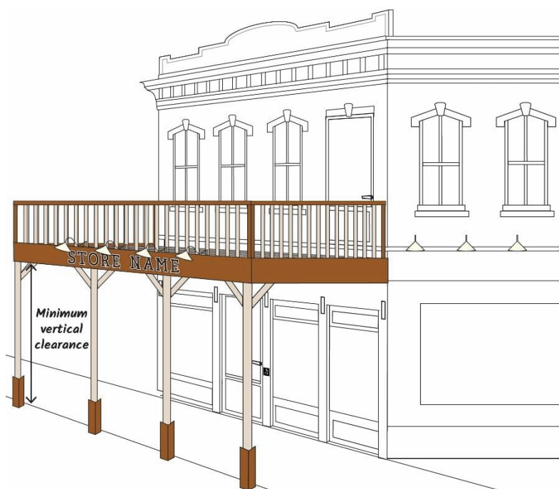
Figure G 2.3.2.6: Accessible Porch with Railings
